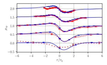
FIG. 8. Lagrangian correlation between streamwise and wall-normal acceleration components. Time delay  $\tau$  is normalized with the local Kolmogorov time scale  $\tau_{\eta}$ . From bottom to top, the curves correspond to particles located initially at  $y_0^+ = 20, 60, 200, 600$ , and 1000. (For details, see Fig. 6.)
