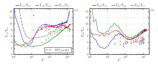
FIG. 12. Lagrangian time scale ratios. Experiments, crosses; DNS, solid lines. (a) Ratio between the Lagrangian velocity and acceleration time scales, by component. Also shown is the HIT model [6] for the ratio of Lagrangian velocity and acceleration time scales. (b) Ratio between the time scales of acceleration magnitude and the components of acceleration.
