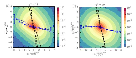
FIG. 15. Joint PDF of streamwise and wall-normal acceleration at  $y^+ = 15$  and 59. Conditional means  $\langle a_x | a_y \rangle / \langle a_x^2 \rangle^{1/2}$  and  $\langle a_y | a_x \rangle / \langle a_y^2 \rangle^{1/2}$  are superposed to the contours using black and blue markers, respectively. Experiments, circles; DNS, dashed lines.
