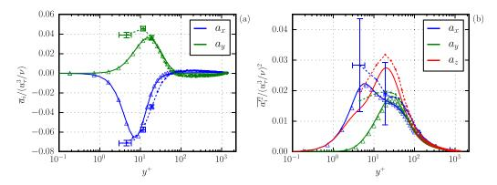
FIG. 4. Mean and variance acceleration profiles. Comparison between experiments (dashed lines), DNS (solid lines), and Yeo *et al.* [30] DNS at Re<sub> $\tau$ </sub> = 600 (triangles).
