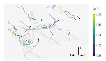
FIG. 1. Sample high-acceleration particle tracks obtained from DNS. Particles are located in the near-wall region ( $y^+ \lesssim 200$ ). Trajectories are shown over  $\Delta t^+ = 120$ . The shadow is projected on the wall. Colors represent the norm of particle acceleration.  $|\mathbf{a}^+| = 1$  corresponds roughly to  $430 \,\mathrm{m/s^2}$  in the experiments.
