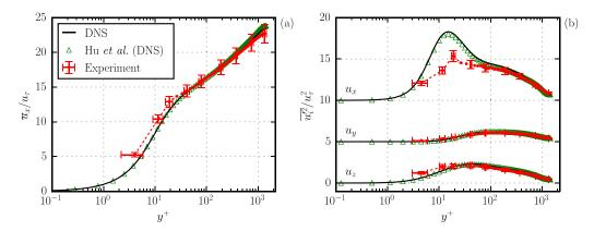
FIG. 3. Mean and variance velocity profiles. Comparison between experiments (dashed lines), DNS (solid lines), and Hu *et al.* [27] DNS at  $Re_{\tau} = 1440$  (triangles). Velocity variance profiles are shifted vertically for clarity. All quantities are normalized in wall units.
