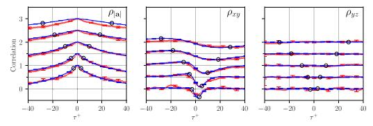
FIG. 7. From left to right, Lagrangian autocorrelation of acceleration magnitude ( $\rho_{|\mathbf{a}|}$ ) and acceleration cross-correlations  $\rho_{xy}$  and  $\rho_{yz}$ . From bottom to top, the curves correspond to particles located initially at  $y_0^+ = 20, 60, 200, 600,$  and 1000. (For details, see Fig. 6.)
