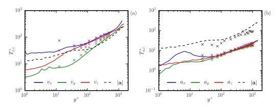
FIG. 10. Lagrangian velocity and acceleration time scales in wall units. Experiments, crosses; DNS, solid lines. The acceleration magnitude time scale  $T_{[a]}$  is represented by dashed lines.
